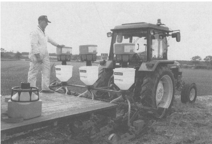
Fig. 12.9 'Sure Fill' closed transfer of granules.
