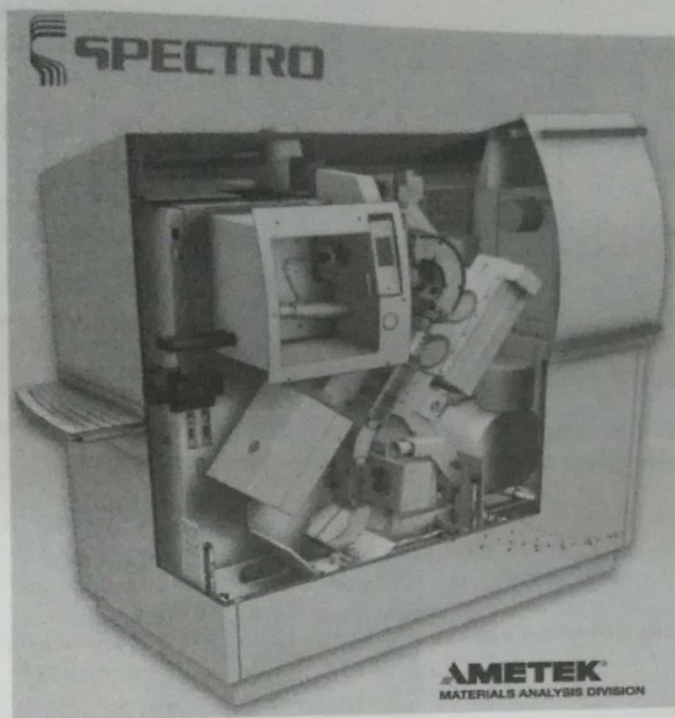
Figure 9.24 Cutaway view of the SPECTRO MS, showing the ICP torch box upper left and the ion optic to the right of the torch box, leading to the mass spectrometer on the left under the torch box. (Courtesy of SPECTRO Analytical Instruments, Inc., AMETEK® Materials Analysis Division. www.spectro.com, www.ametek.com. Used with permission.)
