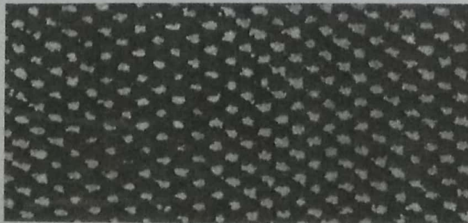
Figure 8.62 An electron micrograph of the (110) plane in crystalline silicon.
