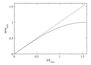
Fig. 16.3 Dispersion of the discrete wave equation
