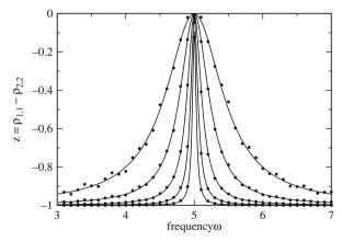
**Fig. 19.14** Power saturation and broadening. The resonance line is investigated as a function of the coupling strength V and compared with the stationary solution (19.171) to observe the broadening of the line width (19.173). Parameters are  $\omega_0 = 5$ ,  $z_{\rm eq} = -1.0$ ,  $T_1 = T_2 = 100$ , and V = 0.5, 0.25, 0.125, 0.0625, 0.03125
