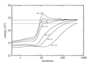
Fig. 15.2 Influence of the relaxation parameter. The convergence of the interaction energy ((15.20), which has a value of 34.56 eV for this example) is studied as a function of the relaxation parameter  $\omega$ . The optimum value is around  $\omega \approx 1.9$ . For  $\omega > 2$  there is no convergence. The dash-dotted line shows the exact value. The dashed line shows the exact value for a corrected radius which is derived from the occupied volume (15.35)
