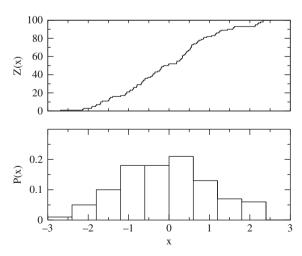
**Fig. 8.3** Histogram. The cumulative distribution of 100 Gaussian random numbers is shown together with a histogram with bin width  $\Delta x = 0.6$
