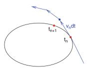
**Fig. 11.2** Systematic errors of the Euler method
