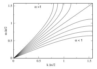
Fig. 16.2 Dispersion of the discrete wave equation. Only for small values of  $k\Delta x$  and  $\omega \Delta t$  is the dispersion approximately linear. For  $\alpha < 1$  only frequencies  $\omega < \omega_{\text{max}} = 2\arcsin(\alpha)/\Delta t$  are allowed whereas for  $\alpha > 1$  the range of k-values is bounded by  $k_{\text{max}} = 2\arcsin(1/\alpha)/\Delta x$
