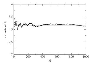
Fig. 8.5 Convergence of the numerical integration
