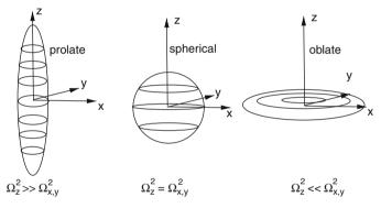
**Fig. 14.6** Gyration tensor. The eigenvalues of the gyration tensor give information on the shape of the polymer. If the extension is larger (*smaller*) along one direction than in the perpendicular plane, one eigenvalue is larger (*smaller*) than the two other
