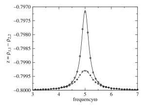
**Fig. 19.13** Resonance line. The equations of motion of the two-level system including relaxation terms are integrated with the fourth-order Runge–Kutta until a steady state is reached. Parameters are  $\omega_0 = 5$ ,  $z_{\rm eq} = -0.8$ , V = 0.01, and  $T_1 = T_2 = 3.0$ , 6.9. The change of the occupation difference is shown as a function of frequency (*circles*) and compared with the steady-state solution (19.171)
