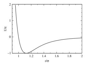
Fig. 13.1 Lennard-Jones potential. The 6–12 potential (13.3) has its minimum at  $r_{\min} = \sqrt[6]{2}\sigma \approx 1.12\sigma$  with  $U_{\min} = -\epsilon$
