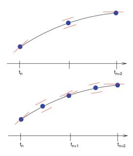
**Fig. 11.7** Step doubling with the fourth-order Runge–Kutta method
