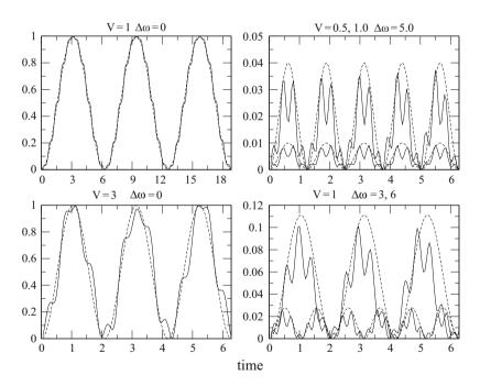
**Fig. 19.12** Simulation of a two-state system in an oscillating field. The equations of motion (19.99) are integrated with the fourth-order Runge-Kutta method. At resonance the system oscillates between the two states with the frequency  $V/\hbar$ . The *dashed curves* show the corresponding solution of a two-level system with constant coupling (Sect. 19.4.2).
