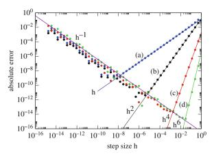
**Fig. 3.2** Numerical differentiation. The derivative  $\frac{d}{dx}\sin(x)$  is calculated numerically using algorithms with increasing error order (3.1(a), 3.7(b), 3.13(c), 3.17(d)). For very small step sizes the error increases as  $h^{-1}$  due to rounding errors
