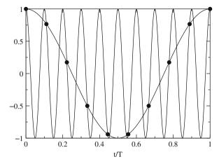
Fig. 7.1 Equivalence of  $\omega_1$  and  $\omega_{N-1}$ . The two functions  $\cos \omega t$  and  $\cos(N-1)\omega t$  have the same values at the sample points  $t_n$  but are very different in between
