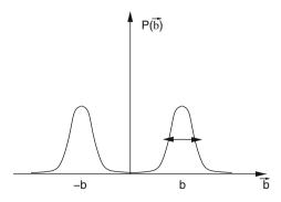
Fig. 14.8 Distribution of bond vectors. The bond vector distribution for a one-dimensional chain of springs has maxima at  $\pm b$ . For large force constants the width of the two peaks becomes small and the chain of springs resembles a freely jointed chain with constant bond length
