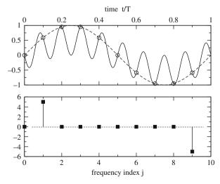
**Fig. 7.2** Trigonometric interpolation. For trigonometric interpolation the high frequencies have to be replaced by the corresponding negative frequencies to provide meaningful results between the sampling points. The *circles* show sampling points which are fitted using only positive frequencies (*full curve*) or replacing the unphysical high frequency by its negative counterpart (*broken curve*). The *squares* show the calculated Fourier spectrum
