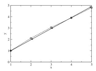
**Fig. 10.1** Linear approximation by singular value decomposition. The data set (10.70) is shown as *circles*. The linear approximation which is obtained by retaining only the dominant singular value is shown by the *squares* and the *solid line*
