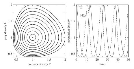
**Fig. 18.8** Lotka–Volterra model. The predator and prey population densities show periodic oscillations (right). In the H-P plane the system moves on a  $closed\ curve$ , which becomes an ellipse for small deviations from equilibrium (left)
