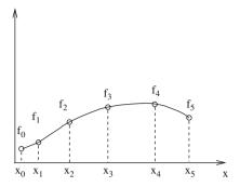
Fig. 2.1 Interpolating function
