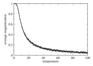
Fig. 13.6 Numerical simulation of the one-dimensional Ising model. The average magnetization per spin is calculated from a MC simulation (*circles*) and compared to the exact solution (13.44). Parameters are  $\mu B = -5$  and J = -2
