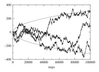
Fig. 14.2 Random walk with constant step size. The figure shows the position  $r_n$  for three different one-dimensional random walks with step size  $\Delta x = \pm 1$ . The *dashed curves* show the width  $\pm \sigma = \pm \sqrt{n}$  of the Gaussian approximation (14.8)
