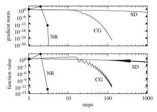
**Fig. 6.5** Stationary points. The minimum of the Rosenbrock function  $h(x, y) = 100(y - x^2)^2 + (1 - x)^2$  is determined with different methods. Conjugate gradients converge much faster than steepest descent. Newton–Raphson reaches the minimum at x = y = 1 within only four iterations to machine precision
