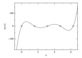
Fig. 2.3 Interpolation error. The polynomial  $\omega(x)$  is shown for the example (2.25). Its roots  $x_i$  are given by the x values of the sample points (*circles*). Inside the interval  $x_0 \dots x_4$  the absolute value of  $\omega$  is bounded by  $|\omega(x)| \le 35$  whereas outside the interval it increases very rapidly
