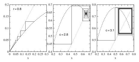
**Fig. 18.5** Orbits of the logistic map. *left:* For 0 < r < 1 the logistic map has the attractive fixed point  $x^* = 0$ . *middle:* In the region 1 < r < 3 this fixed point becomes unstable and another stable fixed point is at  $x^* = 1 - 1/r$ . *right:* For  $3 < r < 1 + \sqrt{6}$  the second-order fixed point (18.33) is stable. For larger values of r more and more bifurcations appear
