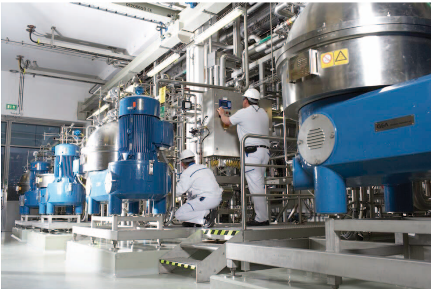
FIGURE 1.12 Part of an industrial plant for the production of human insulin from genetically engineered Escherichia coli bacteria. (Photo by Felix Denis. With permission from Sanofi-Aventis.)
