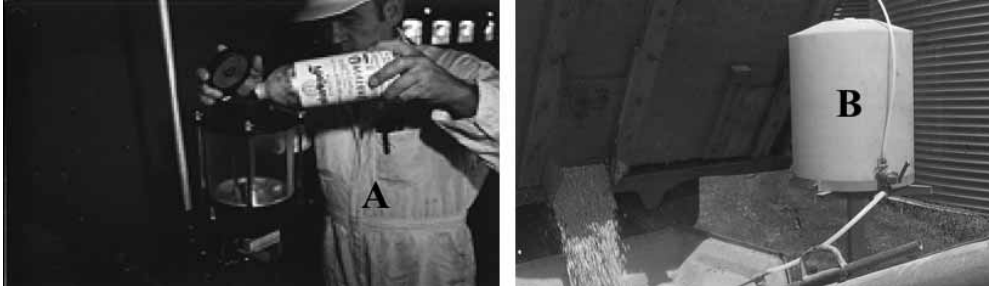
Figure 8. In commercial facilities grain is fumigated by placing phosphine pellets in a pellet dispenser (A). Grain can be treated with a protectant as it is being augered into a bin (B).
