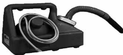
Figure 1. Portable dry powder duster used in solid state disinfection
