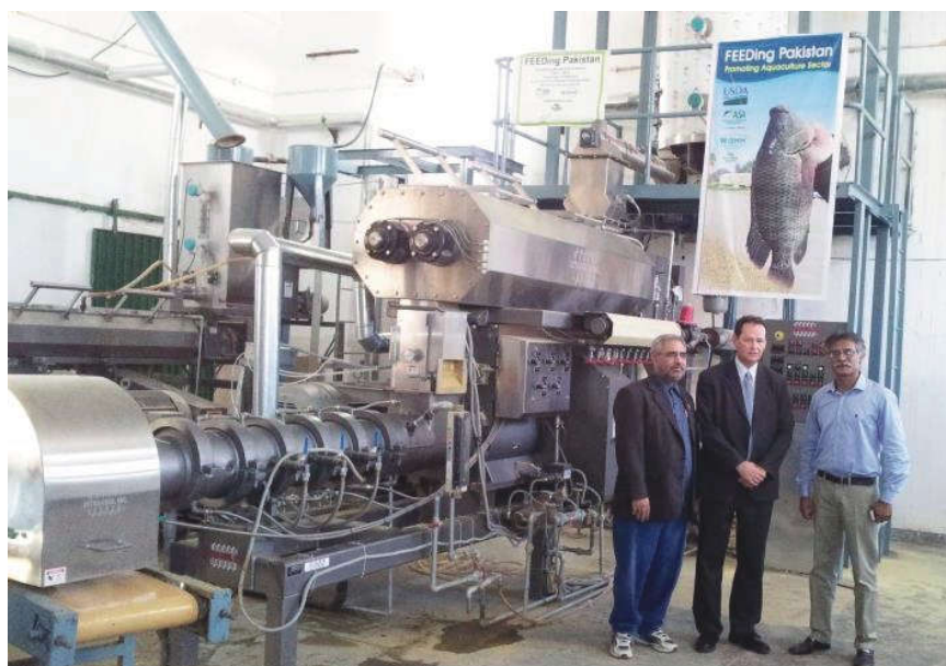
Figure 6. E-750 extruder machine with accessories.
