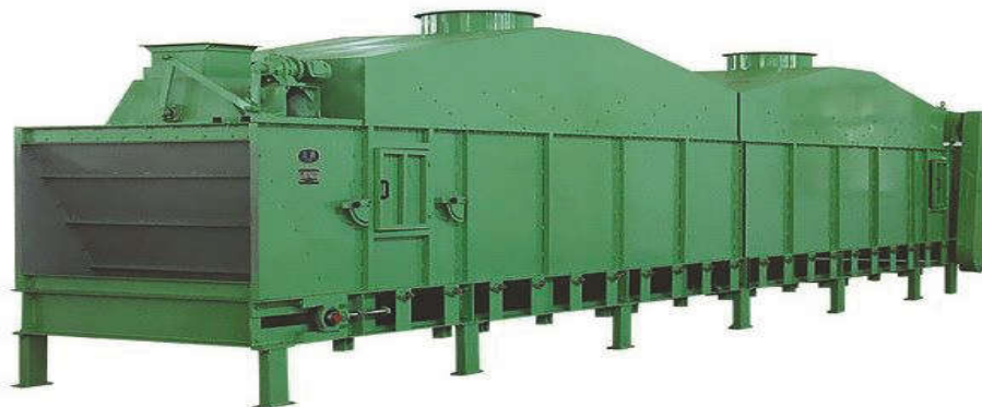
Figure 11. A horizontal belt cooler
