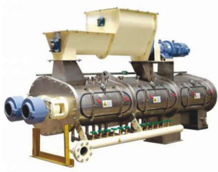
Figure 9. A pre-conditioner with feed hopper
