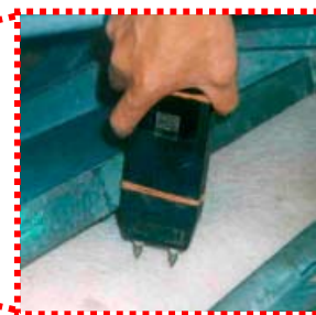
Fig. 6: A battery-operated electric prod
