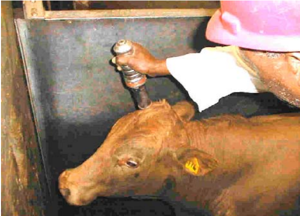
Fig. 53: Hand-held barrel captive bolt gun
