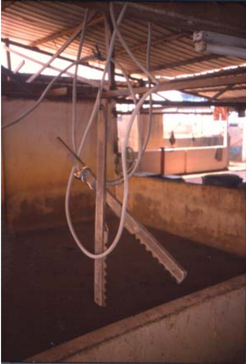
Fig. 70: Makeshift electric stunning tongs
