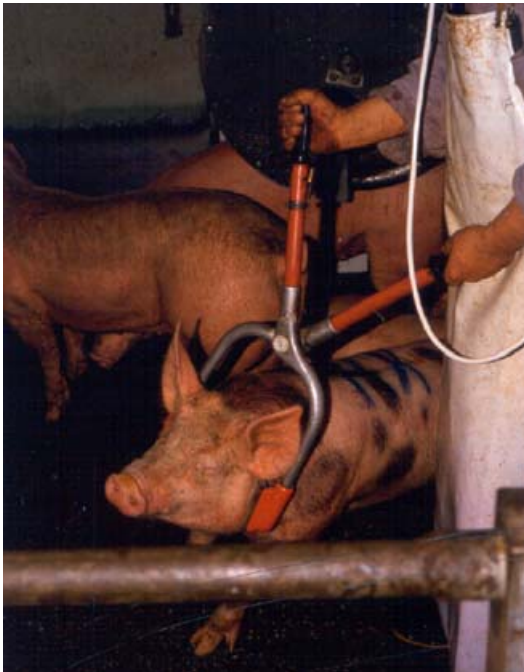
Fig. 57: Tongs for electrical stunning of pigs
