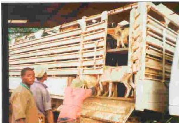
Fig.32: Double-deck truck for transporting sheep/goats
