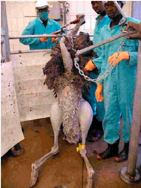
Fig. 59: Tongs for electrical stunning of ostriches
