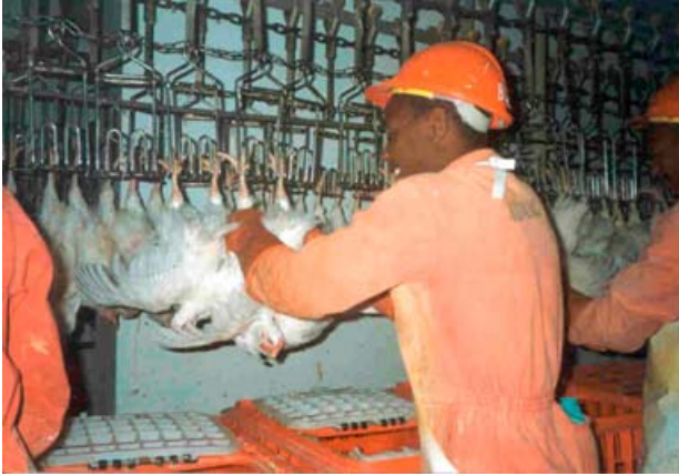
Fig. 49: Poultry shackled on conveyor by legs prior to electric stun
