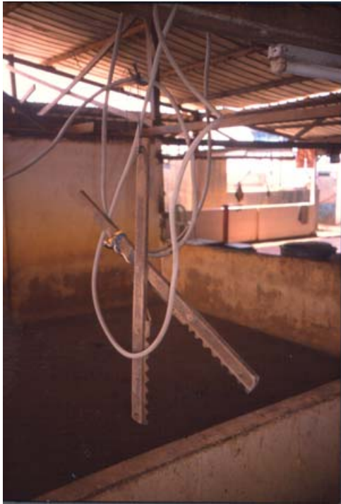
Fig. 70: Makeshift electric stunning tongs
