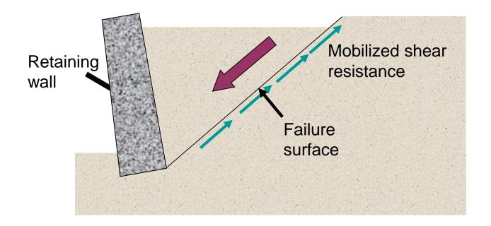
At failure, shear stress along the failure surface (mobilized shear resistance) reaches the shear strength.
