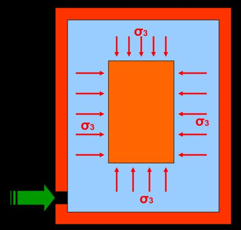
Apply a specific pressure using water
