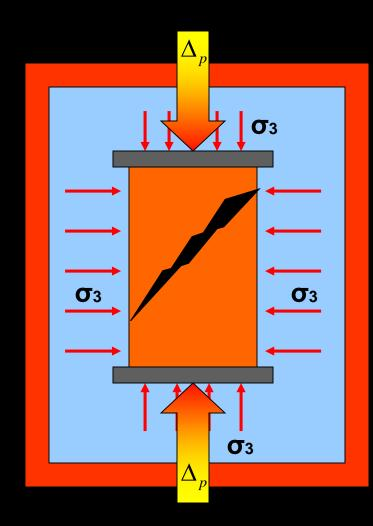
Apply a vertical load and increase until the specimen fails
