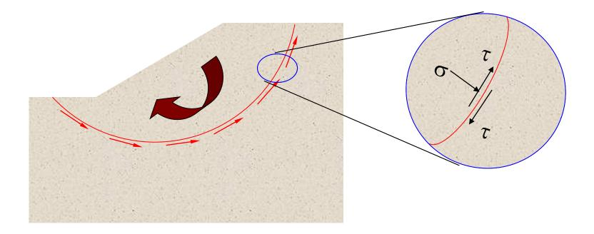
At failure, shear stress along the failure surface reaches the shear strength.
