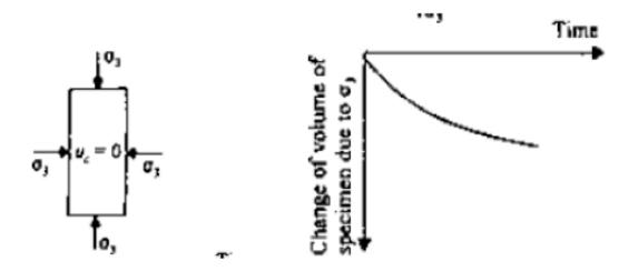
After complete dissipation of excess *pwp*,  $u_c$ , generated by the confining pressure, the deviator stress,  $\Delta \sigma$  is increased to cause failure of the specimen. During this phase of loading, the drainage line from the specimen is closed. Since drainage is not permitted, the *pwp* due to deviator stress,  $u_d$  in the specimen increases. Simultaneous measurements of  $\Delta \sigma$  and  $u_d$  are made during the test.
