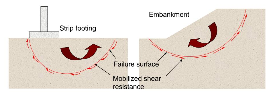
At failure, shear stress along the failure surface (mobilized shear resistance) reaches the shear strength.
