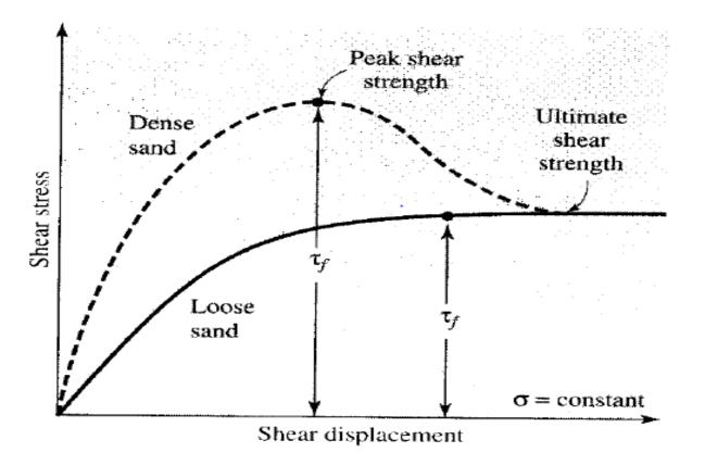
• In dense and medium sand shear stress increases with increase in shear displacement and reaches the maximum or peak value and then decreases to approximate constant value. This point when it become constant is known as ultimate shear strength. However in case of loose sand it increases to maximum value and become constant.
