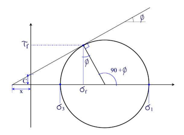
The radius of the circle is  $r = (\sigma_1 - \sigma_3)/2$ The projection of the failure line is  $x=c/tan\phi$
