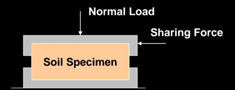
Shear stress = Shearing Force / the specimen's cross- sectional area
