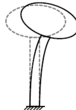
deflected water tower
