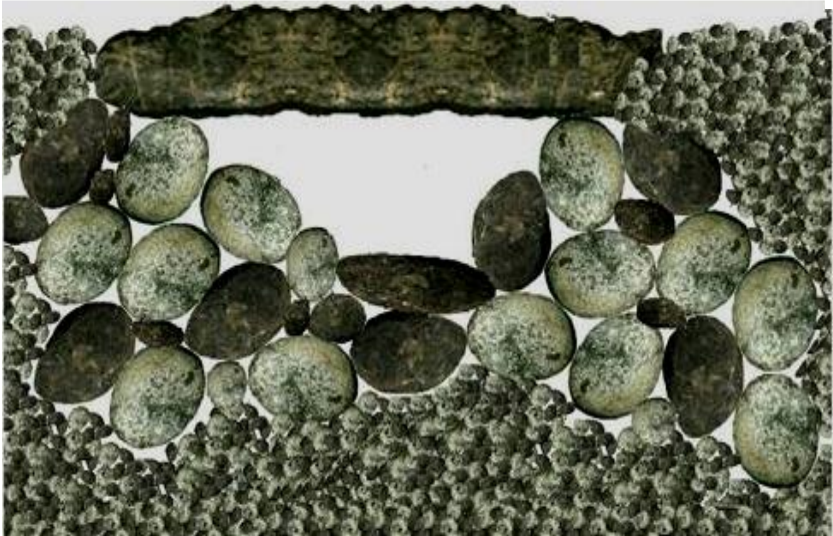
Figure 6: Elongated Particles Bridging a Gap
