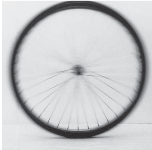
Figure 11-5 A photograph of a rolling bicycle wheel. The spokes near the wheel's top are more blurred than those near the bottom because the top ones are moving faster, as Fig. 11-4c shows.
