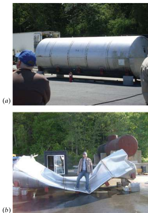
Figure 19-1 (a) Before and (b) after images of a large steel tank crushed by atmospheric pressure after internal steam cooled and condensed.
