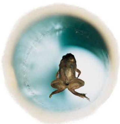
Figure 32-13 An overhead view of a frog that is being levitated in a magnetic field produced by current in a vertical solenoid below the frog.
