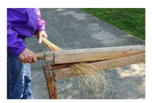
"Scutching". The process separate the unwanted woody matter from fibers. This is also done by beating the straw with blunt wooden or metal blades on the scotching machine. The woody matter is removed as shave, which is usually burnt as fuel, leaving the flax in the form of the long strands formed of bundles of individual fibers adhering to one another.
