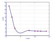
Figure 2: Cubic Hermite Spline Interpolation
