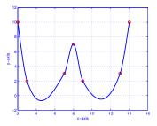
Figure 1: Cubic Hermite Spline Interpolation
