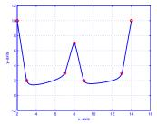
Figure 3: Positive Rational Cubic Spline [5] with  $r_i = w_i = 0.1$
