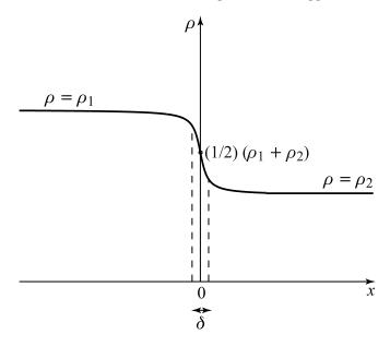
Figure 13.10.1 Shock structure and shock thickness.
