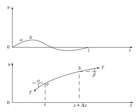
Figure 3.2.1 An Element of a vertically displaced string.
