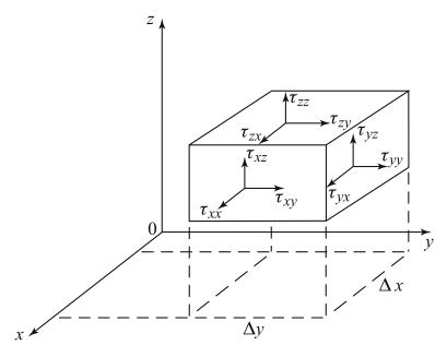
Figure 3.4.1 Volume element of an elastic body.
