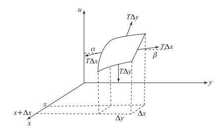
Figure 3.3.1 An element of vertically displaced membrane.
