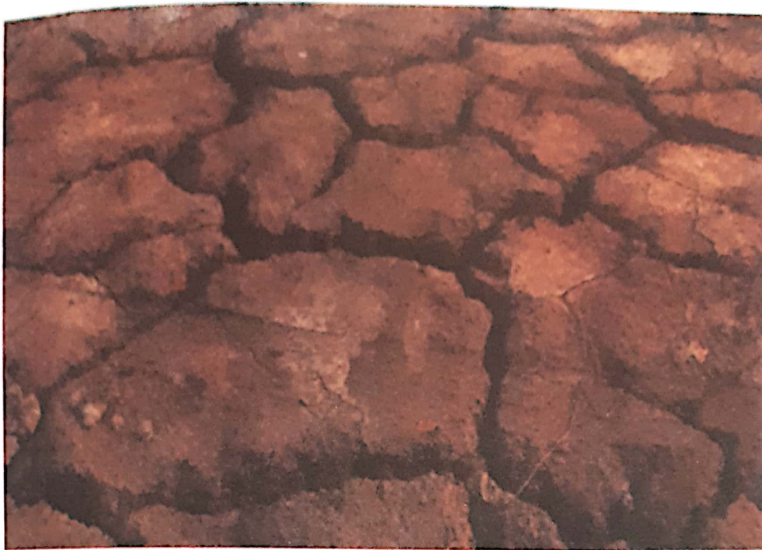
Fig. P-30. Shrinkage cracks at bottom of the Rawal lake which has dried due to severe drought.
