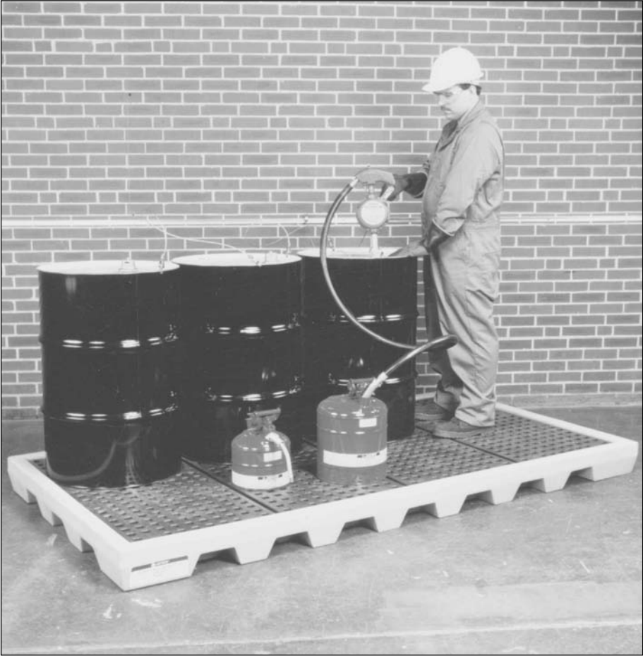
Figure 15-1. Example of a hazardous material accumulation/dispensing center with spill containment.
