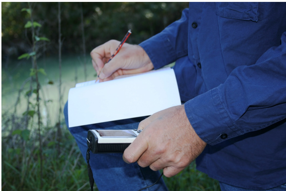
Figure 7. Record the latitude and longitude of the site using a GPS unit. Alternatively, mark your position on a map, and record the grid reference.
