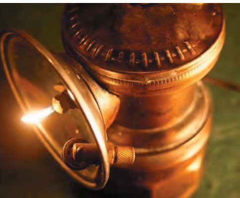
A miner's carbide lamp. Water in the upper chamber slowly drips onto calcium carbide in the lower chamber, generating acetylene.
