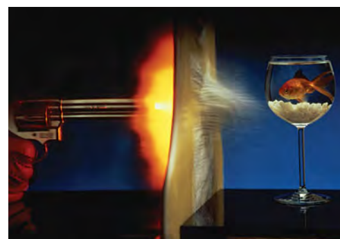
Kevlar ® body armor works by "catching" a bullet in a multilayer web of woven fabrics. Kevlar's extraordinary strength resists tearing and cutting, allowing the stressed fibers to absorb and disperse the impact to other fibers in the fabric.
