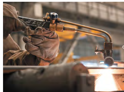
An oxygen–acetylene flame is hot enough to melt steel for welding. A cutting torch uses an extra jet of oxygen to burn away hot steel.
