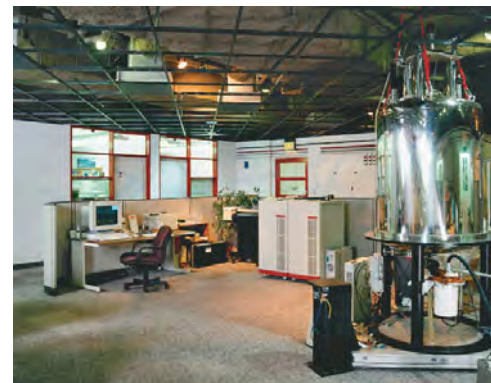
Photo of a modern 300-MHz NMR spectrometer. The metal container at right contains the superconducting magnet, cooled by a liquid helium bath inside a liquid nitrogen bath. The electronics used to control the spectrometer and to calculate spectra are at left and in the background.
