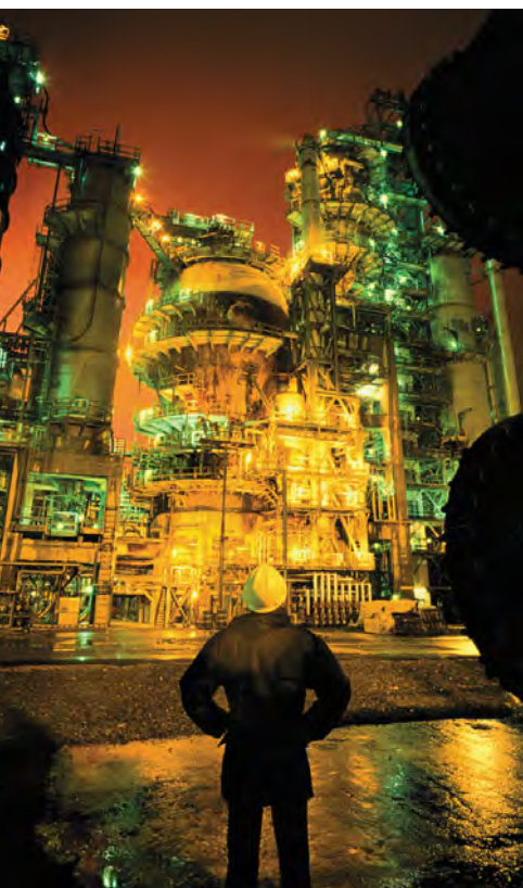
The large distillation tower at left is used to separate petroleum into fractions based on their boiling points. The “cat cracker” at right uses catalysts and high temperatures to crack large molecules into smaller ones.
