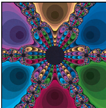
FIGURE 4.53 This computer-generated initial value portrait uses color to show where different points in the complex plane end up when they are used as starting values in applying Newton's method to solve the equation z^6 - 1 = 0 . Red points go to 1, green points to (1/2) + (\sqrt{3}/2)i , dark blue points to (-1/2) + (\sqrt{3}/2)i , and so on. Starting values that generate sequences that do not arrive within 0.1 unit of a root after 32 steps are colored black.
