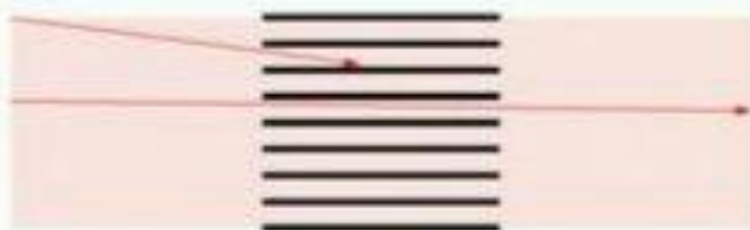
Primary Optics – Soller Slits Axial Divergence
