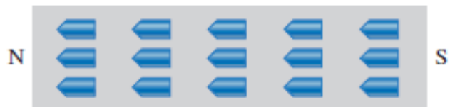
(b) The magnetic domains become aligned when the material is magnetized.
