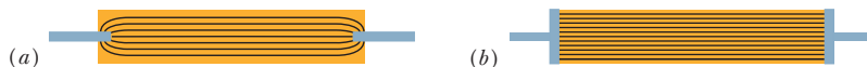
Figure 26-8 Two ways of applying a potential difference to a conducting rod. The gray connectors are assumed to have negligible resistance. When they are arranged as in (a) in a small region at each rod end, the measured resistance is larger than when they are arranged as in (b) to cover the entire rod end.
