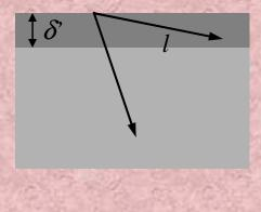
Only electrons moving inside the skin depth for most of the mean free path  $\ell$  are capable of picking up much energy from the electric field. Only a fraction of the electrons  $\delta'/\ell$  contribute to the conductivity
