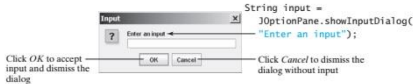
FIGURE 2.5 The input dialog box enables the user to enter a string.
