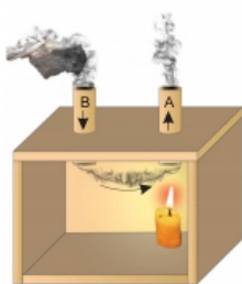
Figure 9.8: Smoke showing the path of the convection.
