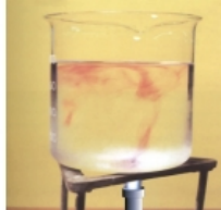
Figure 9.7: Crystals of potassium permanganate are used to show the movement of water on heating.
