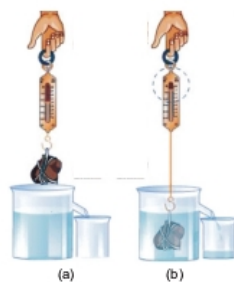
Figure 7.19: (a) weighing solid in air (b) weighing solid in water and measuring water displaced by the solid.
