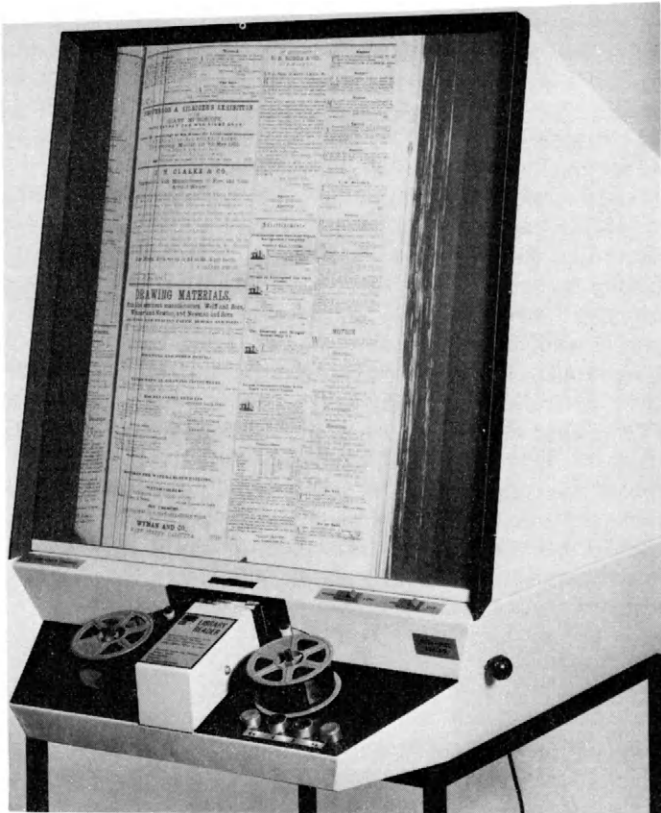
Figure 3.2 Large format microform reader (Allen)
