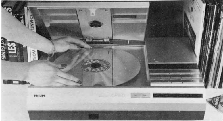
Figure 8.3 Laser disc player (Philips)
