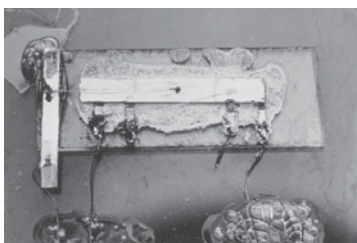
The first integrated circuit, a phase-shift oscillator, invented by Jack S. Kilby in 1958. (Courtesy of Texas Instruments.)
