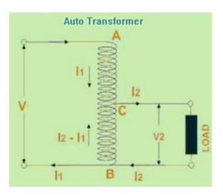
On a single common coil which forms both primary and secondary winding in which voltage is varied according to the position of secondary tapping on the body of the coil windings.
