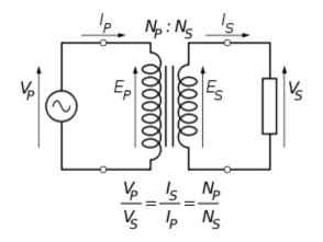
If the secondary coil is attached to a load that allows current to flow, electrical power is transmitted from the primary circuit to the secondary circuit. Ideally, the transformer is perfectly efficient. All the incoming energy is transformed from the primary circuit to the magnetic field and into the secondary circuit. If this condition is met, (i.e, in Ideal transformer) the input electric power must equal the output power:
