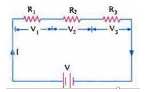
Then the voltage drop through each resistor are  $V_1 = IR_1$ ,  $V_2 = IR_2$  and  $V_3 = IR_3$ . The sum of these voltage drops must be equal to the applied voltage.
