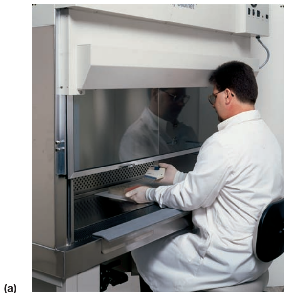
Figure 7.8 A Laminar Flow Biological Safety Cabinet. (a) A technician pipetting potentially hazardous material in a safety cabinet. (b) A schematic diagram showing the airflow pattern.
