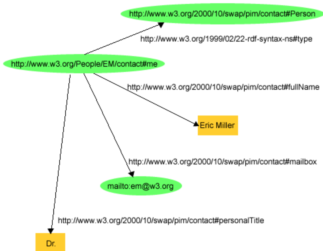
Figure 11 An RDF graph describes Semantic Web innovator Eric Miller through a combination of literal strings and URIs.
