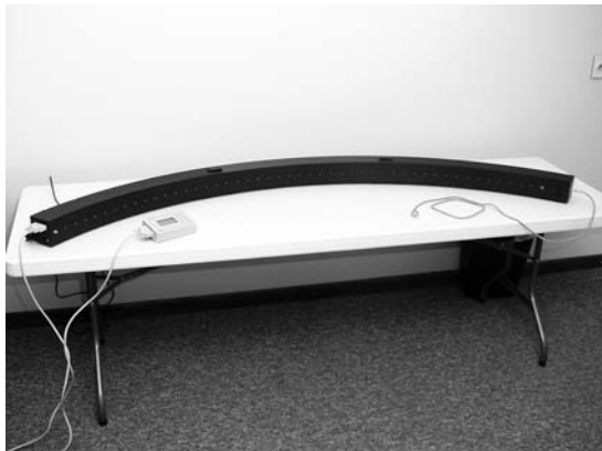
FIGURE 10.36 ▼ Reaction time measuring instrument. (Photo courtesy of Lafayette Instrument Co.)
