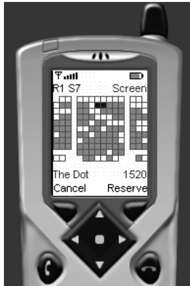
Figure 3.5 Java Smart Ticket Sample Application Displaying an Editable Seating Plan for a Particular Movie Showing
