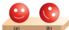
Figure 4.37: Neutral equilibrium (a) a ball is placed on a horizontal surface (b) the ball remains in its new displaced position.
