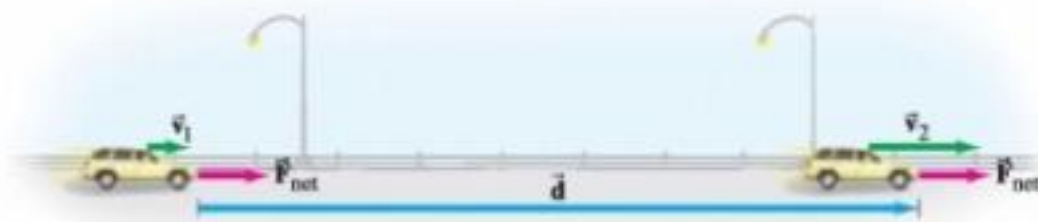
FIGURE 7-14 A constant net force F_{\text{net}} accelerates a car from speed v_1 to speed v_2 over a displacement d . The net work done is W_{\text{net}} = F_{\text{net}}d .
