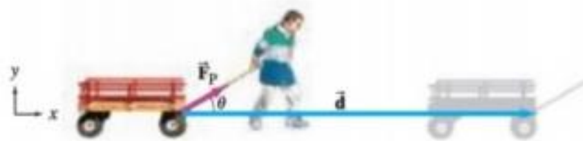
FIGURE 7-7 Example 7-4. Work done by a force \vec{F}_p acting at an angle \theta to the ground is W = \vec{F}_p \cdot \vec{d} .
