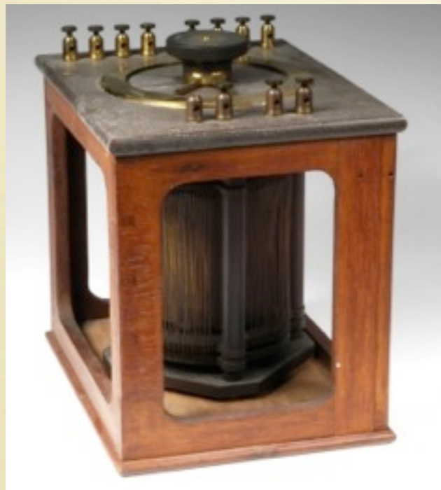
Marconi Bellini-Tosi Direction Finder Designed for detecting the positions of enemy wireless stations
