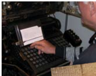
Linotype machine used to create newspapers in days of hot metal by Stephen Quinn
