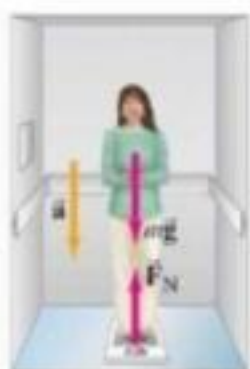
FIGURE 4-17 Example 4-8. The acceleration vector is shown in gold to distinguish it from the red force vectors.
