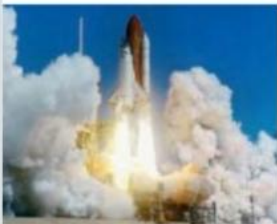
FIGURE 4-10 Another example of Newton's third law: the launch of a rocket. The rocket engine pushes the gases downward, and the gases exert an equal and opposite force upward on the rocket, accelerating it upward. (A rocket does not accelerate as a result of its propelling gases pushing against the ground.)
