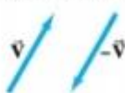
FIGURE 3-7 The negative of a vector is a vector having the same length but opposite direction.
