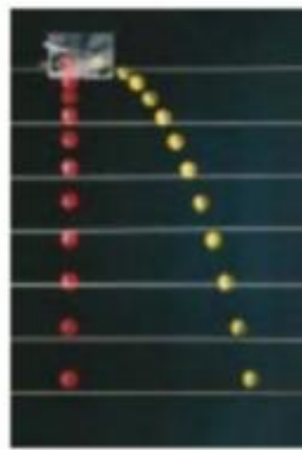
FIGURE 3-21 Multiple-exposure photograph showing positions of two balls at equal time intervals. One ball was dropped from rest at the same time the other was projected horizontally outward. The vertical position of each ball is seen to be the same at each instant.
