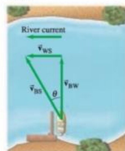
FIGURE 3-34 Example 3-15. A boat heading directly across a river whose current moves at 1.20 m/s.
