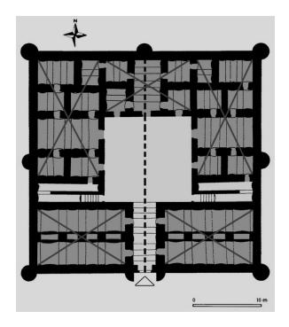
**Figure 1:** Plan of Kharana Umayyad desert palace, as a model illustrating the interior layout space distribution, division, the *bayts* units and symmetry (After Haddad:2009, fig.5).
