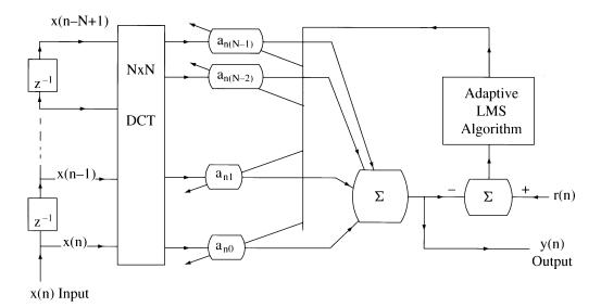
FIGURE 3.7 Adaptive transform domain LMS filtering.
