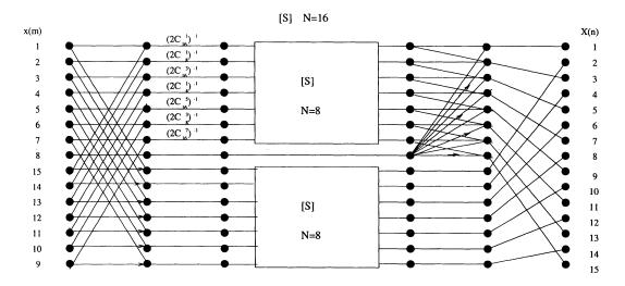
**FIGURE 3.15** DIF DST N = 16 flow graph  $\rightarrow (-1)$ .
