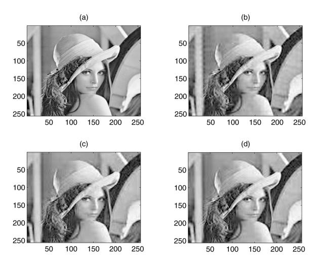
**FIGURE 3.11** Comparisons of original and reconstructed image, M = L = 16, at 0.16 bpp: (a) original at 8 bpp, (b) DLS, (c) LOT, (d) MLT.
