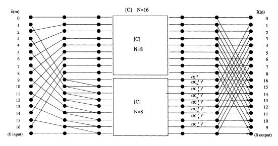
**FIGURE 3.12** DIT DCT N = 16 flow graph  $\rightarrow (-1)$ .
