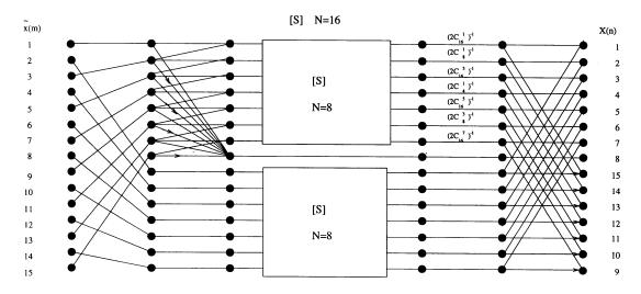
**FIGURE 3.13** DIT DST N = 16 flow graph  $\rightarrow (-1)$ .
