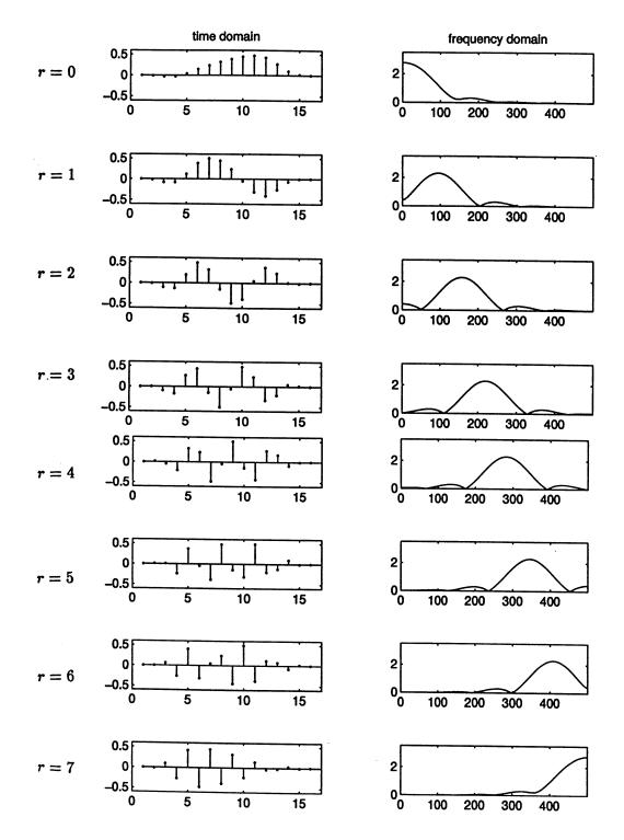
**FIGURE 3.8** DLS basis functions in time and frequency domain, L = M = 8.
