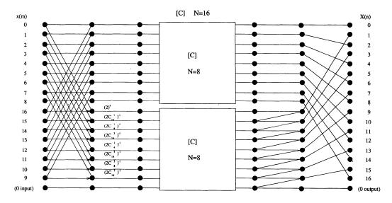
**FIGURE 3.14** DIF DCT N = 16 flow graph  $\rightarrow (-1)$ .
