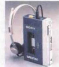
This walkman is powered by batteries of the primary cell type. Typically, they have to be replaced every two or three months.
