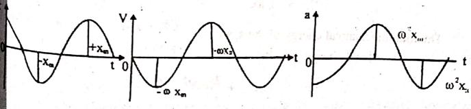
The graph shows magnitude of maximum displacement of simple harmonic ator is  $x_m$ . The magnitude of maximum velocity is  $\omega x_m$  while magnitude of mum acceleration is  $\omega^2 x_m$ .
