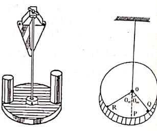
Rotate the disc in horizontal plane through angle  $\theta_m$  such that reference line OP reaches at line OQ. The wire gets twisted and torque is produced. The line OQ on disc moves towards reference line OP when wire is allowed to untwist. The twisting of wire creates a restoring torque. The line OP oscillates between OQ and OR under this restoring torque.
