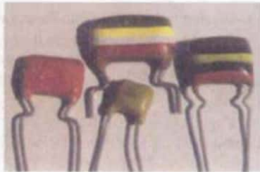
Fig. 5.27. The small value ceramic capacitors.
