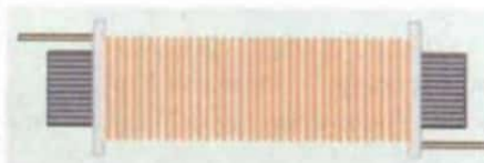
Laminated iron cores are generally used in low cost, low power inductors.
