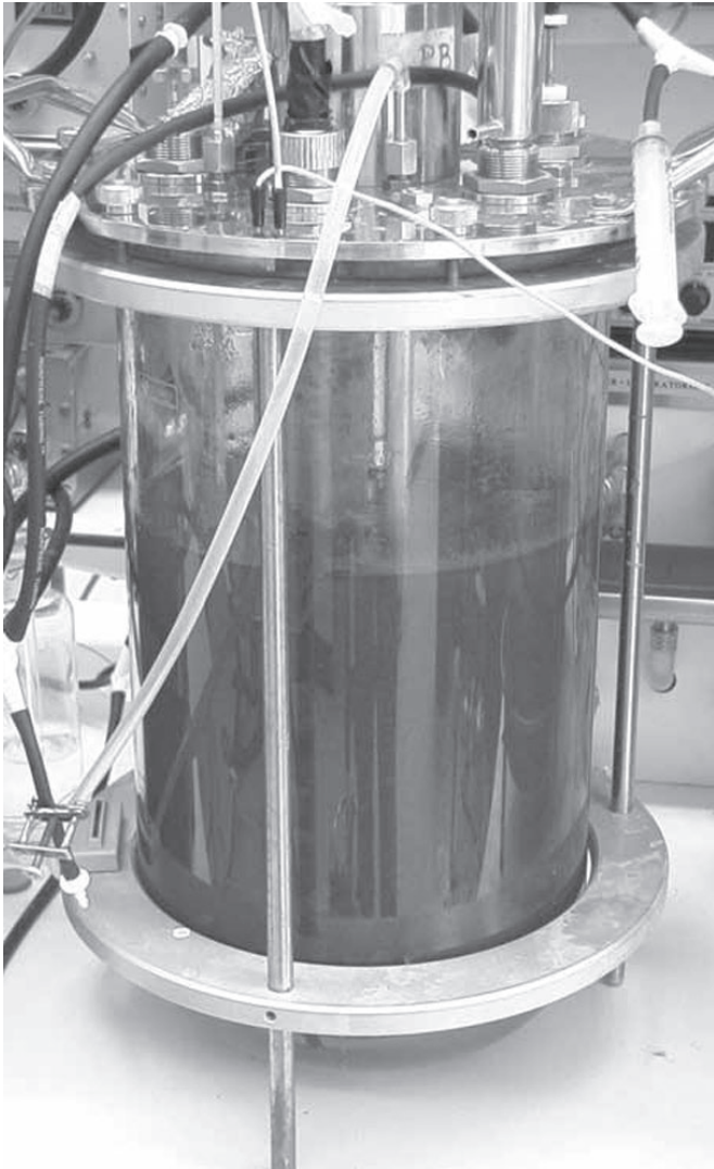
FIGURE 12 Bioreactor Containing Candidatus Brocadia anammoxidans , Anaerobic Bacterium That Can Degrade Ammonium Novel metabolic properties enable these anaerobes to degrade ammonium from wastewater in a single step.
