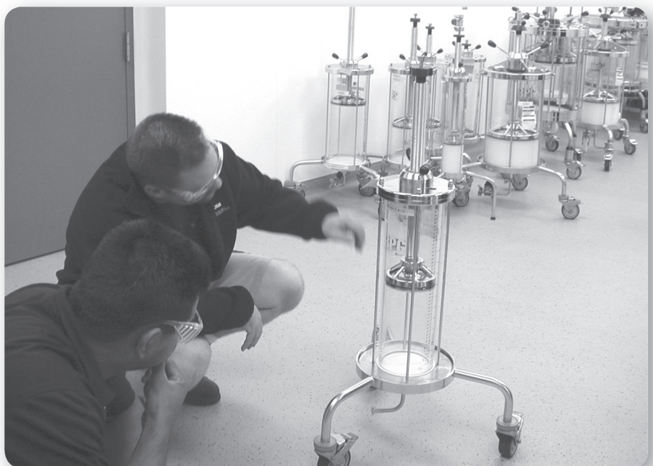
Lab Supervisor Preparing a Purification Column to Separate a Commercial Biological Product.
