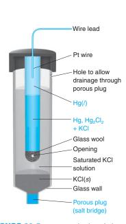
**FIGURE 14-5** A saturated calomel electrode (S.C.E.).
