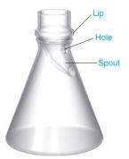
FIGURE 27-11 Reflux cap for wet ashing in an Erlenmeyer flask. The hole allows vapor to escape. The curved spout touches the inside of the flask. [From D. D. Siemer and H. G. Brinkley, "Erlenmeyer Flask-Reflux Cap for Acid Sample Decomposition," *Anal. Chem.* **1981**, *53*, 750.]
