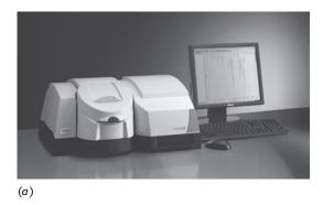
FIGURE 19-3 (*a*) Thermo Scientific Evolution 600 ultraviolet-visible double-beam spectrophotometer. (*b*) Optical train of Evolution 600, showing layout of components. [Courtesy Thermo Fisher Scientific, Madison, WI.]
