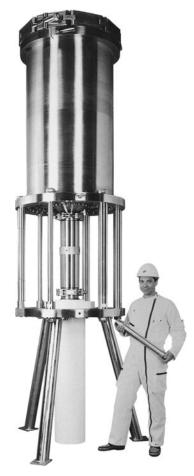
FIGURE 22-8 Industrial-scale preparative chromatography column can purify a kilogram of material. The column volume is 300 L. [Courtesy Prochrom, Inc., Indianapolis, IN.]
