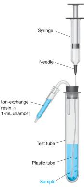
FIGURE 27-20 Apparatus for trapping basic or acidic gases by ion exchange. [From D. D. Siemer, "Ion Exchange Resins for Trapping Gases: Carbonate Determination," *Anal. Chem.* **1987**, *59*, 2439.]
