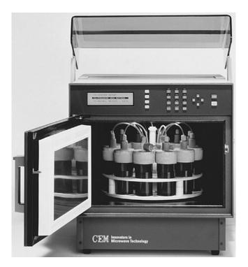
FIGURE 27-12 Extraction vessels in a microwave oven that processes up to 12 samples in under 30 min. Each 100-mL vessel has a vent tube that releases vapor if the pressure exceeds 14 bar. Vapors from the chamber are ultimately vented to a fume hood. The temperature inside each vessel can be monitored and used to control the microwave power. [Courtesy CEM Corp., Matthews, NC.]
