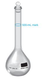
**FIGURE 1-3** A volumetric flask contains a specified volume when the liquid level is adjusted to the middle of the mark in the thin neck of the flask. Use of this flask is described in Section 2-5.
