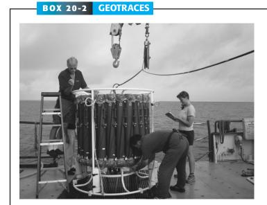
A carousel of 12-L plastic bottles lowered on a Kevlar line from a research vessel is used to collect ocean water without introducing trace metal contamination during collection. Samples are removed from the bottles in a plastic-lined clean room inside a cargo container on the deck of the ship. [Courtesy Gregory A. Cutter, Old Dominion University, Norfolk, VA.]
