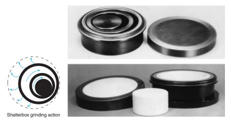
**FIGURE 27-6** Shatterbox laboratory mill spins a puck and ring inside a container at high speed to grind up to 100 mL of sample to a fine powder. [Courtesy Spex Industries, Edison, NJ.]
