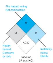
**FIGURE 2-2** Chemical hazards label used by the National Fire Protection Association.
