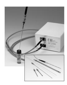
**FIGURE 18-22** Fiber-optic sensor measures  $O_2$  by its ability to quench the luminescence of Ru(II) at the tip of the fiber. A blue-light-emitting diode provides excitation energy. Inset shows several probes. [Courtesy Ocean Optics, Dunedin, FL.]
