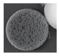
FIGURE 24-5 Scanning electron micrograph of 4.4-µm-diameter microporous silica chromatography particle from an experimental batch made by K. Wyndham at Waters Corporation. [Photo kindly provided by J. Jorgensen, University of North Carolina.]
